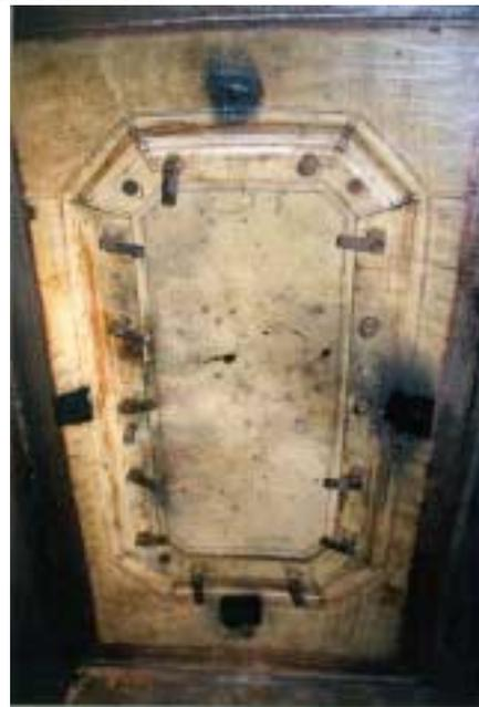
**Figure 23** The Prima Membrane Mk3 door in the DERA Blast Test box (Post Trial).
