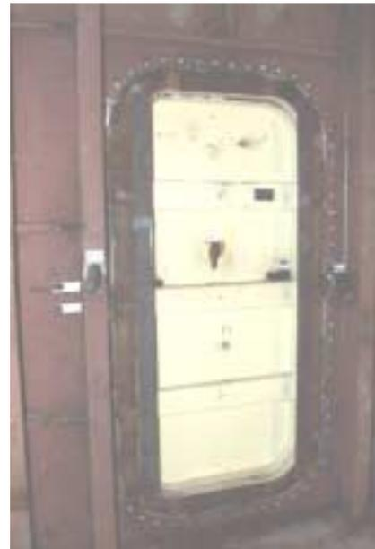
**Figure 13 A level I door in its test frame**
