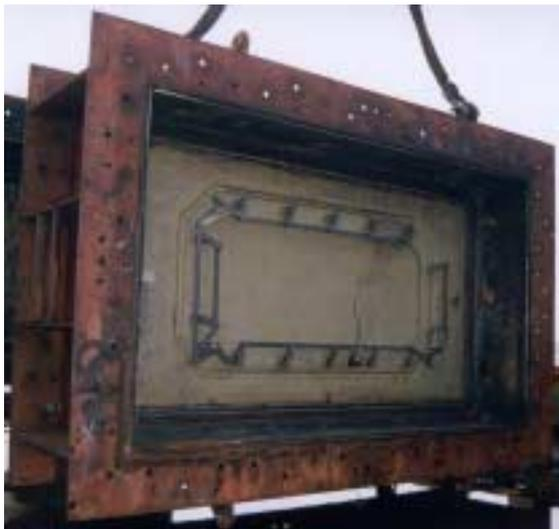
**Figure 22** The Prima Membrane Mk3 door in the DERA Blast Test box (Pre Trial).
