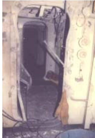
*Figure 11 A Roofdier Trial Result; WT-doors taken out by the detonation of a medium sized naval shell.*
