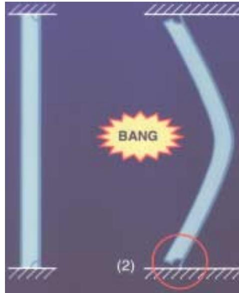
*Figure 10 High Stress and Strain at the BHD & Deck connection*
